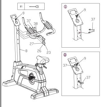
Step 4 Attach the handlebar mast to the frame assembly. Remove the screws from the joint of frame and handlebar. Put the upper shroud (21) on the handlebar mast. Connect the motor cables and console cables (9) and (22). Attach the console mast to frame assembly. Then tighten the hex screws, flat washers and spring washers. Attach the handlebar mast to the frame assembly.
